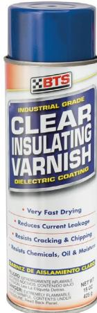
BTS Industrial Grade Clear Insulating Varnish is formulated to protect, seal and insulate surfaces against deterioration from exposure to oil, moisture, acid and alkali. BTS B-00066 provides a high gloss air drying enamel barrier recommended for use as a finish coat for Class "F" winding or electrical apparatus.
